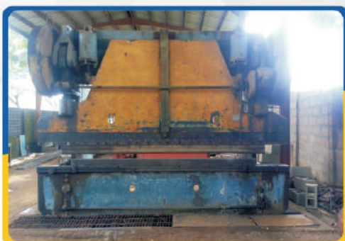
Bending Machine 12mm X 5m Capacity
