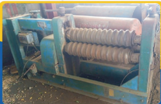
CORRUGATED STEEL ROLLER
