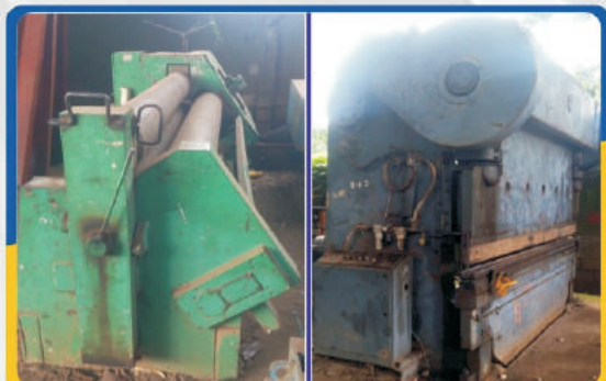
ROLLING MACHINE 10MM X 2.5 CAPACITY
