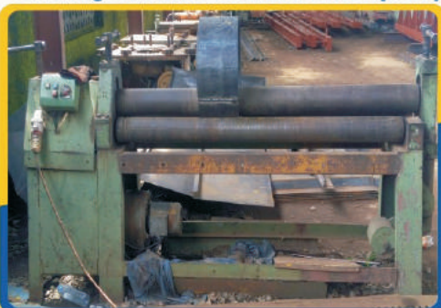
Rolling Machine 20mm X 2.5m Capacity
